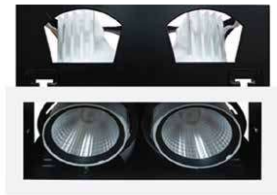
OPL-MATRIX-M2/30 OPL-MATRIX-M2/40 LED 10Wx2 3600lm (3000K 4000K) W14.7 x L26.4 x H11.7
